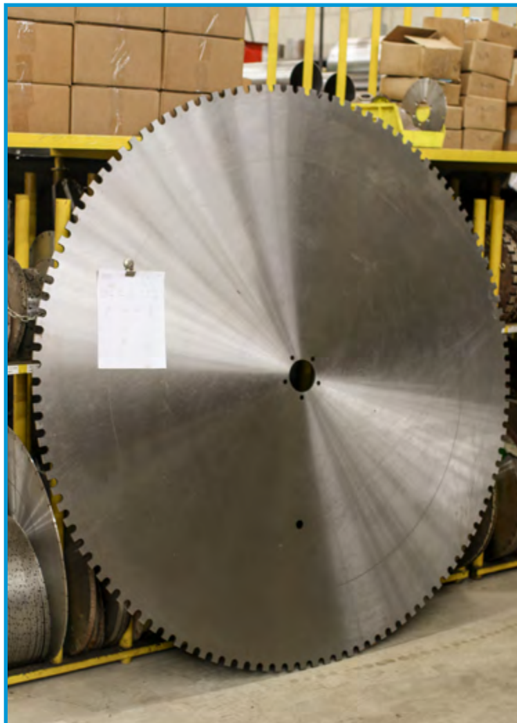
Below and right: 60 inch block saw blade, and retipped blades
