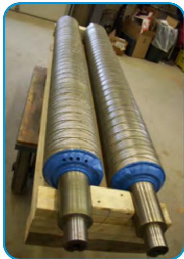
8-foot surface milling tools custom-developed for processing and leveling Indiana Limestone slabs.
