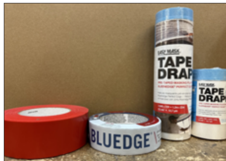
Red tape, blue tape, 24 and 48 inch wide Tape & Drape – essentials needed for almost every restoration job.
