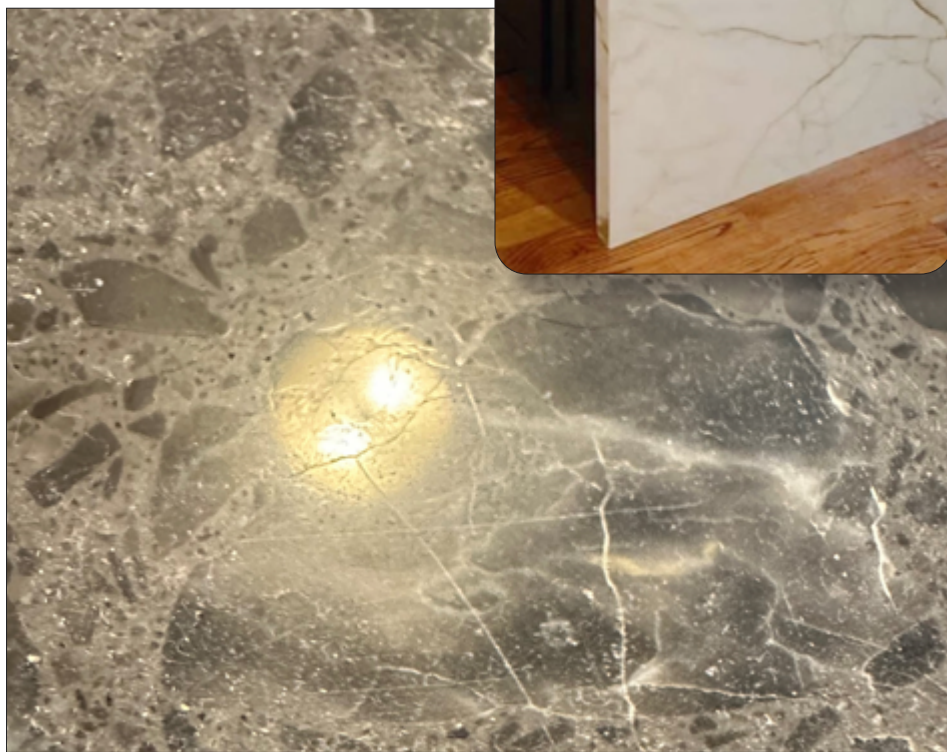
Engineered marble. Note the minor surface scratches.
