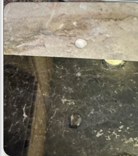
A drop of hydrochloric acid on marble (top picture) and on granite. Note that on the marble, the acid effervesces, and on the granite the acid has no reaction.
