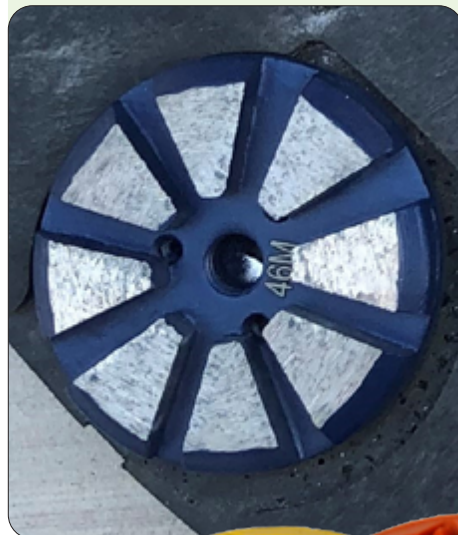
Segmented metal bond MAGNUM MAG3- 0400 grit mounted on a GRIP magnetic plate, closeup, below.
