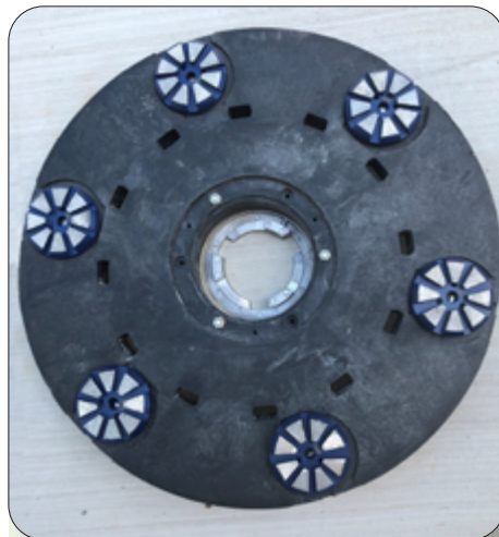
Segmented metal bond MAGNUM MAG3- 0400 grit mounted on a GRIP magnetic plate, closeup, below.
