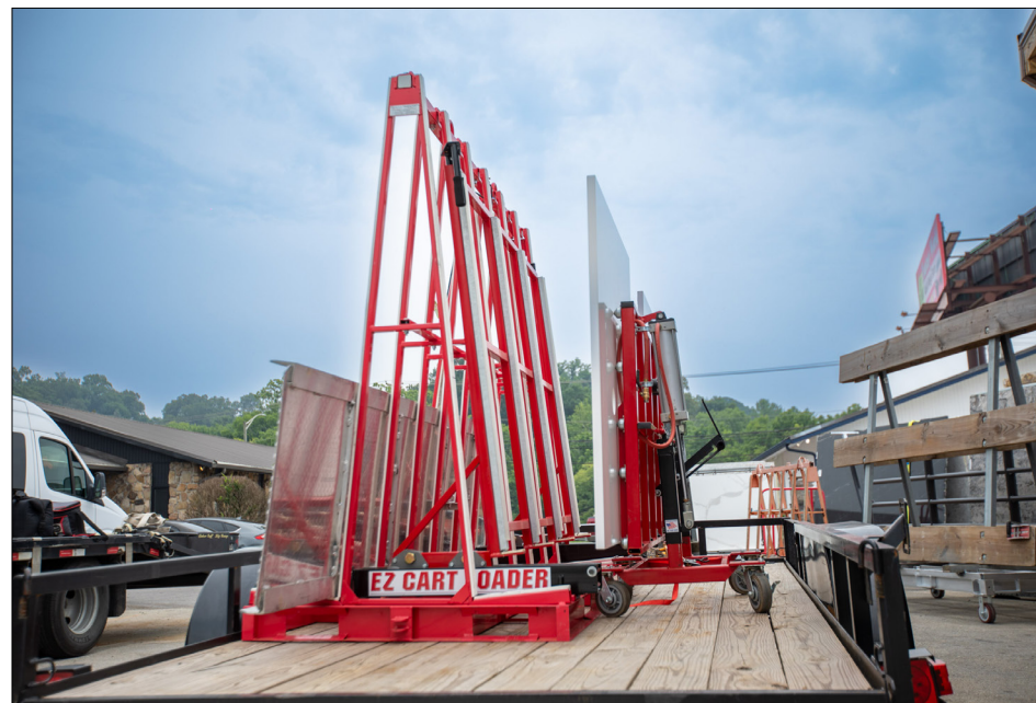
Starting at the shop: loading a large island top from EZ Installation Cart to a transport cart.
