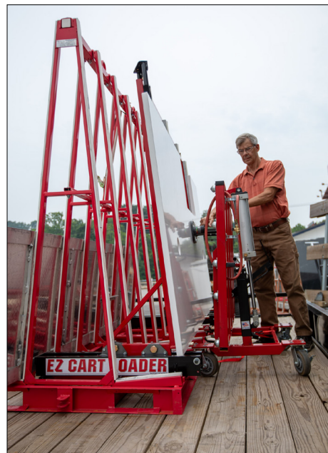
Transferring a large island top from a transport cart to the EZ Installation Cart, can almost effortlessly be done by one person.
