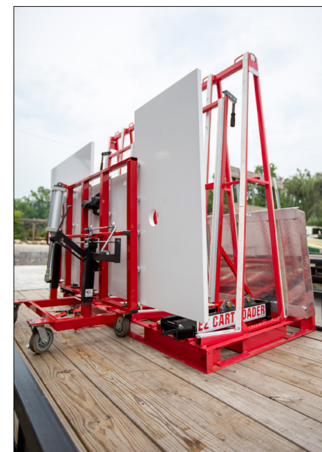
Island top loaded and ready to roll into the jobsite with the EZ Installation Cart.
