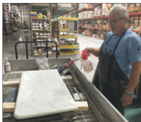
Here I'm using a small pump-up sprayer as the water source for refinishing an antique marble vanity top.
